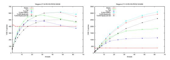
**Figure 4.** Throughput of the randomized work distribution benchmark on a 64 thread Niagara II. On the left a small array of 60K locations and a pattern of strong intra-transaction spatial locality and on the right 500K locations with moderate intra-transaction spatial locality. Sets of 32 locations are read and then written in these arrays.
