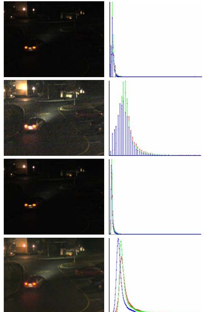
Figure 10: Inspection of color histograms in our process. From top to bottom: the original video frame and its histogram; a histogram stretched frame and its histogram showing quantization error; an ASTA processed frame and its histogram which is similar to the unfiltered histogram; the tone mapped ASTA frame and its stretched histogram without quantization error. Note the vertical scale in these histograms is vertically stretched to show maximum detail in each.
