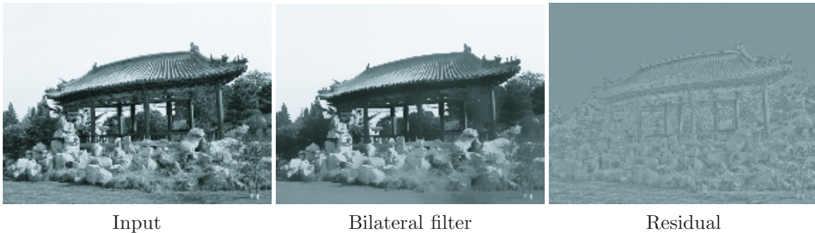
Figure 8: Separation: The residual of the bilateral filter reveals the structure of the input image: Ideally for denoising tasks, the residual should contain only noise. Nonetheless, the structure visible in the residual is faint and bilateral filtering yields acceptable results in numerous denoising scenarios.
