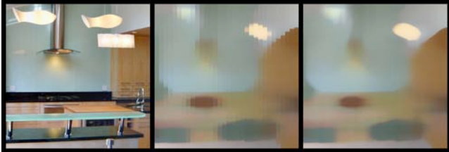
Figure 7: Pivot Tracking. The middle image shows the approximation obtained using one pivot per sixteen columns to track the smallest median values. H^* is then scanned upwards from these pivots (several columns at a time, vectorized) to yield the exact median result, right.
