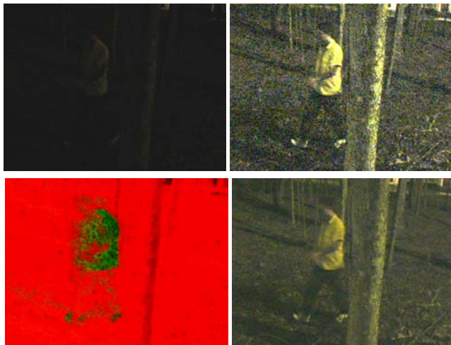
Figure 8: A frame from a video processed using virtual exposures. Upper Left: original frame; Upper Right: histogram stretched version; Bottom Left: red = number of temporal pixels integrated, green = number of spatial pixels integrated; Bottom Right: our result after filtering and tone mapping.
