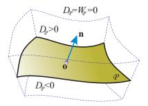
**Figure 2.** The patch  $\mathcal{P}$ . The dashed lines delimit the neighborhood.  $\mathbf{o}$  is the center of  $\mathcal{P}$ , and  $\mathbf{n}$  the local estimation of the normal.
