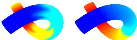
**Figure 10:** Penalizing curvature often leads to fuzzy boundaries (left), the opposite more quickly isolates the part in conflict and propagates a frontier that respects the feature (right).
