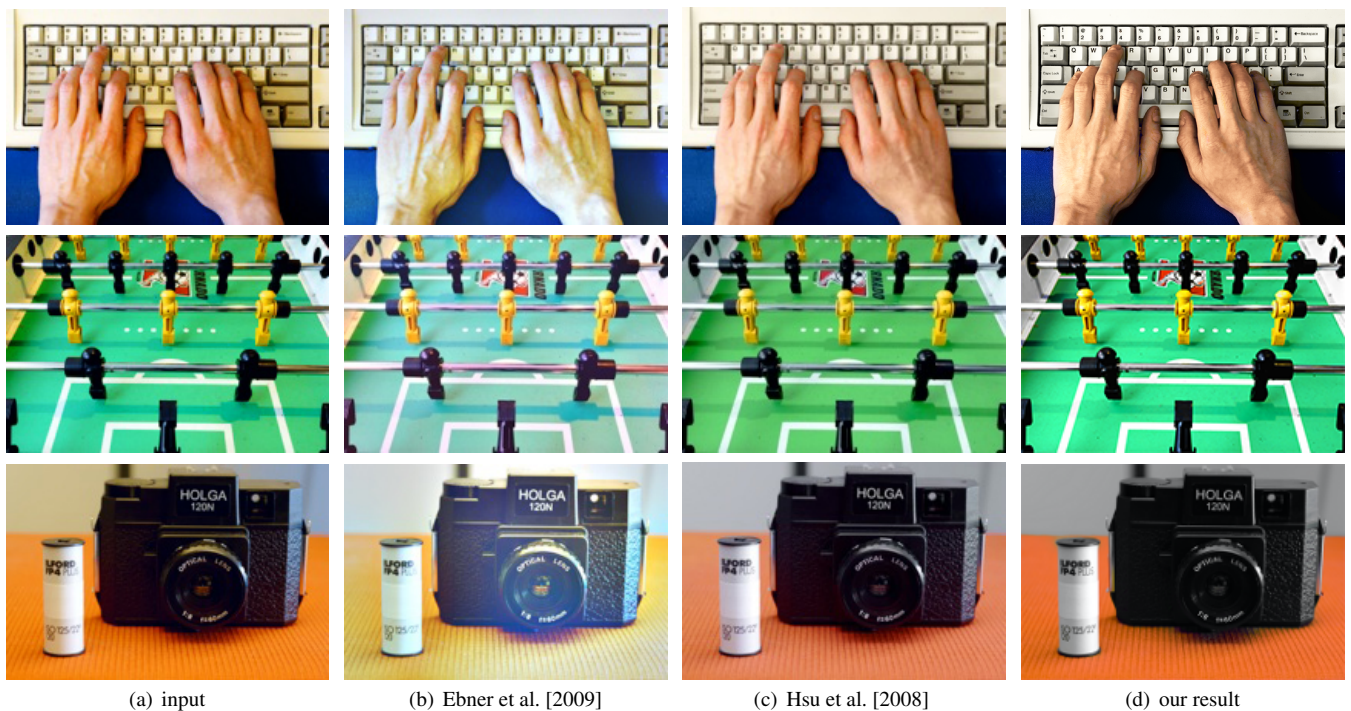
Figure 10: Comparison for images from Hsu et al. [2008] (a). Ebner’s method [2009] tends to produce desaturated results (b). These results are reproduced from Ebner et al. [2009]. Hsu et al. [2008] (c) and our method (d) produce equivalent results with no color cast. The two approaches differ in that Hsu et al. is automatic but assume two lights of known colors, whereas our method is user-assisted and does not make assumptions about the illumination. The results by Hsu et al. are reproduced from their article.
