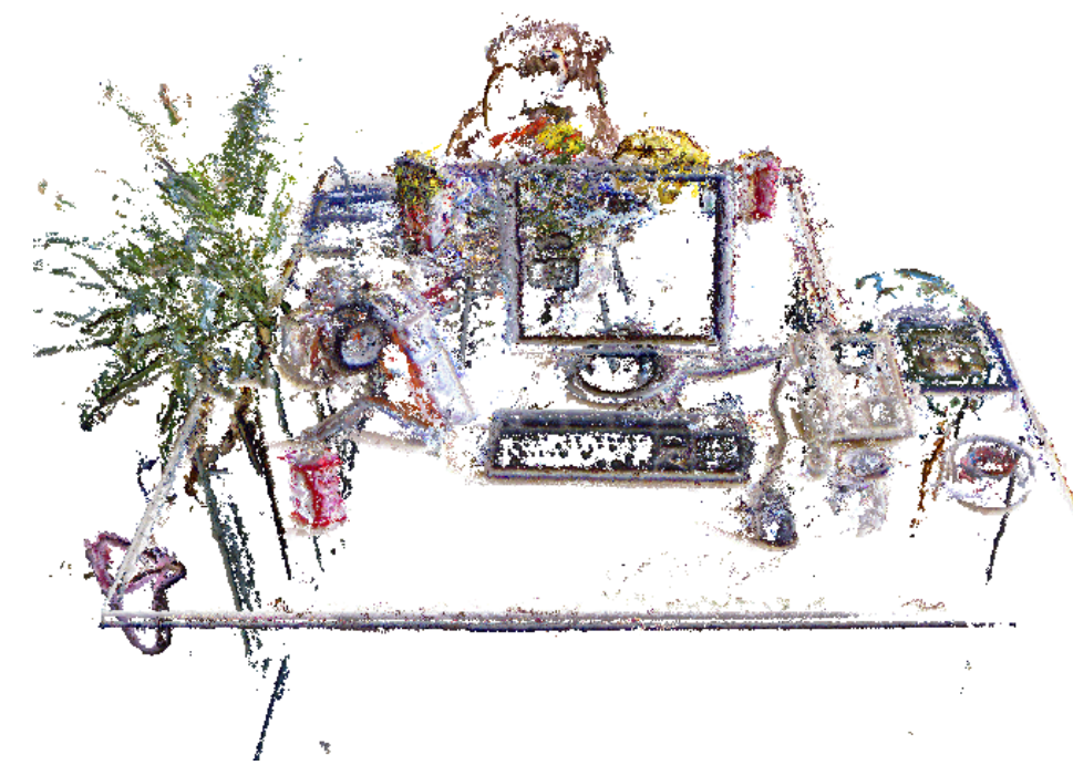
Semi-Dense Mapping with ORB-SLAM Mur-Artal et al. (RSS 2015)
