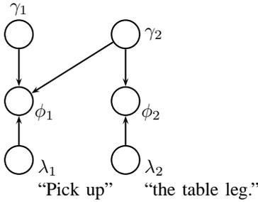
Fig. 3. Grounding graph for the command, “Pick up the table leg.” Random variables and edges are created in the graphical model for each constituent in the parse tree. The  $\lambda$  variables correspond to language; the  $\gamma$  variables correspond to groundings in the external world. Edges in the graph are created according to the parse structure of the command
