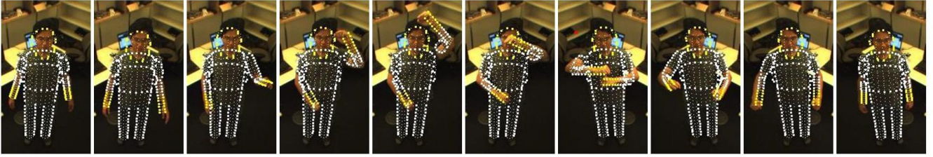
Figure 5. Sample image sequence with the estimated body pose superimposed on the user in each frame.
