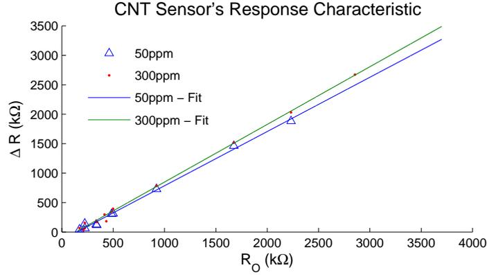
Figure 1-7: The sensor characteristic showing the proportionality of  $\Delta R$  to  $R_{base}$  [3]
