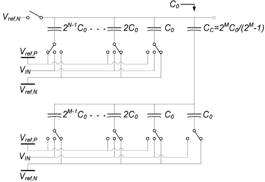
Figure A-1: The concept of sub-DAC implementation [6]
