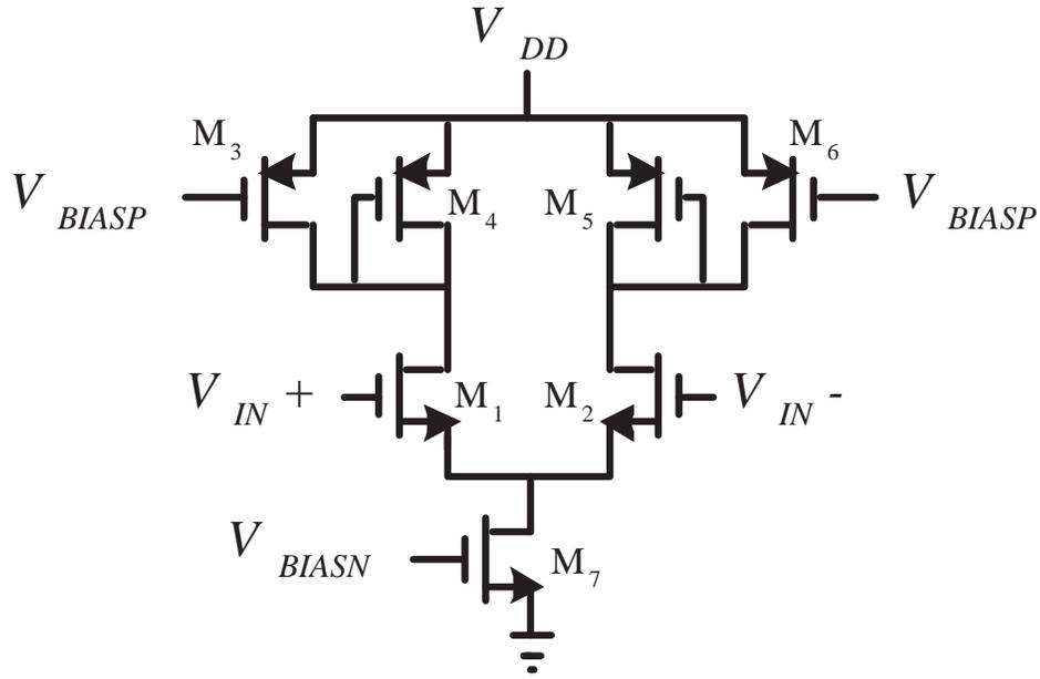
Figure 3-4: The preamplifier used in the comparator
