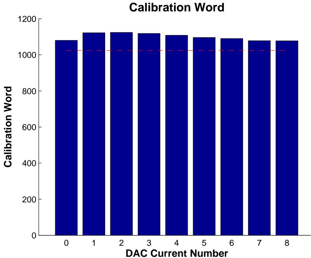
Figure 4-5: Calibration words for the given measurements. The red line denotes the unity gain points
