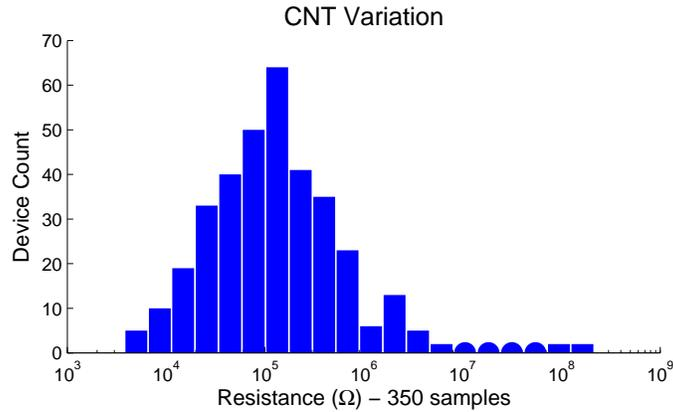
Figure 1-4: Local variation of CNT resistance due to poor process controls [3]
