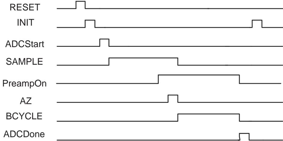
Figure 3-2: Control sequence for the designed SAR ADC
