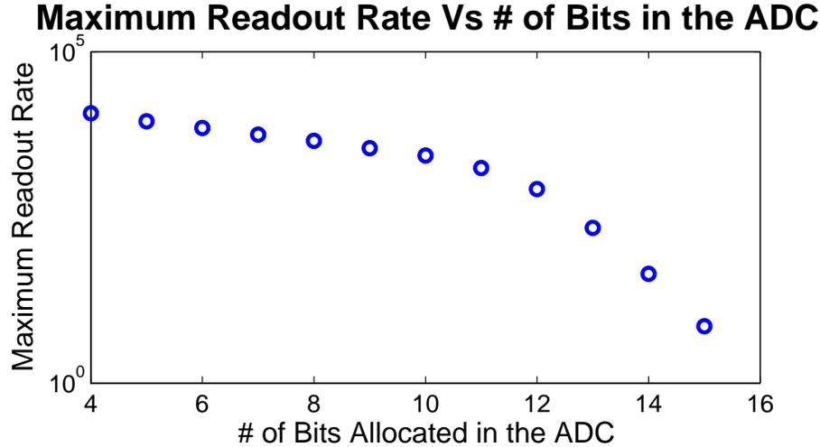
Figure 2-9: Sensing rate changes as ADC resolution varies
