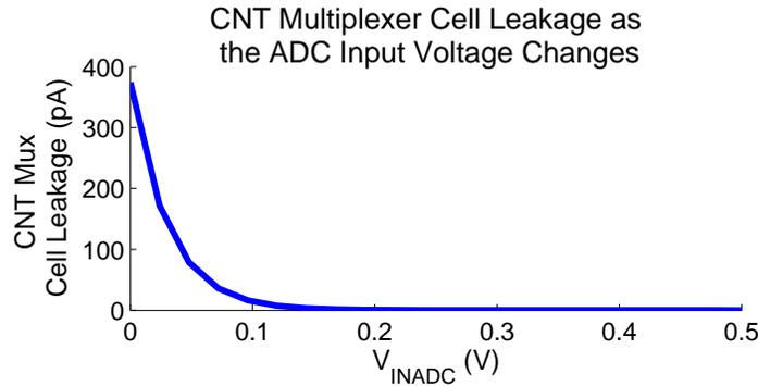
Figure 3-16: The leakage characteristic of a multiplexer cell as the  $V_{INADC}$  is varied.
