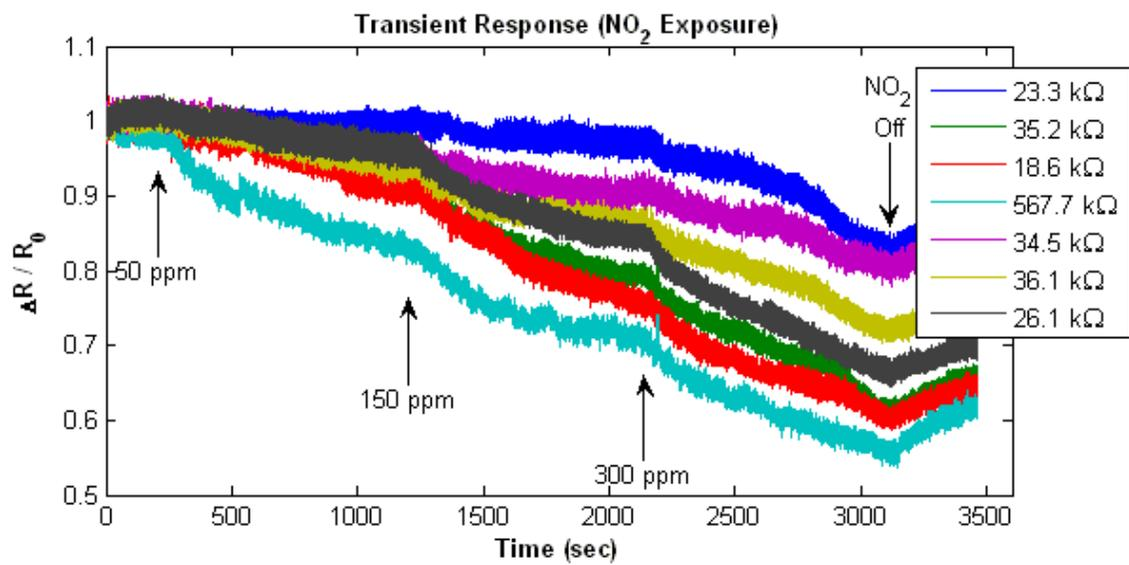
Figure 4-12: The resistance of CNTs changes when exposed to different concentrations of  $NO_2$
