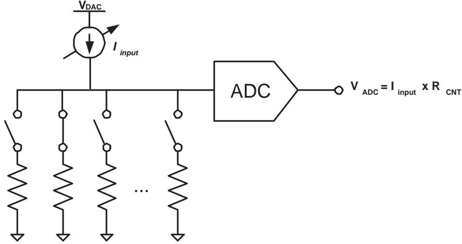
Figure 2-4: Basic idea of the proposed architecture
