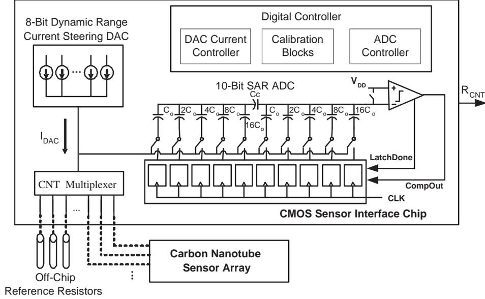
Figure 2-5: The proposed system architecture
