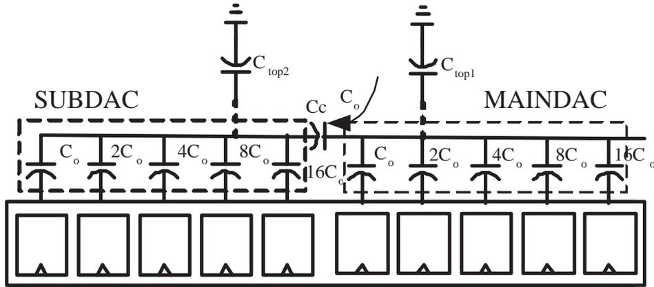
Figure 3-10: The configuration of capacitive DAC implemented for the ADC. Note the illustration of the top plate parasitics.
