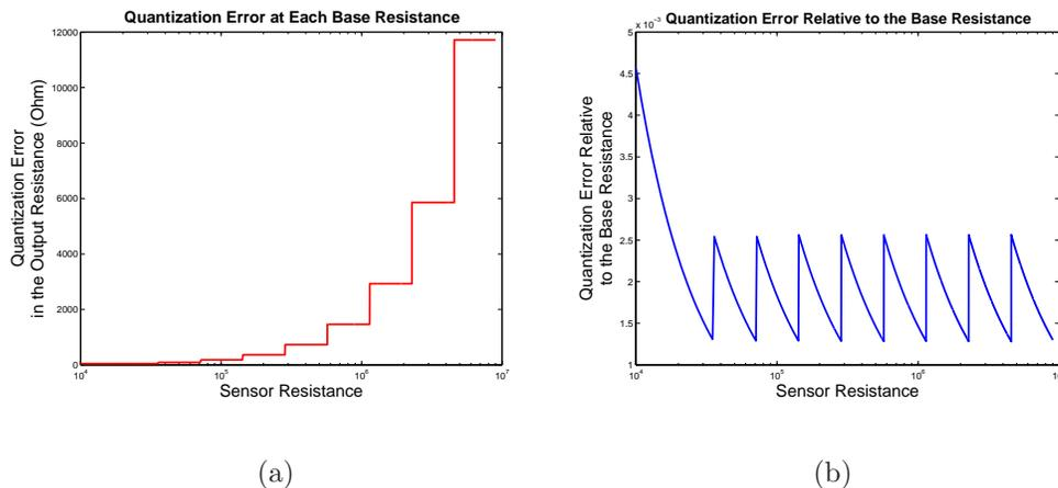
Figure 2-12: Figure 2-12(a) shows the absolute quantization error at each resistance level, and Figure 2-12(b) shows the quantization error relative to each resistance level
