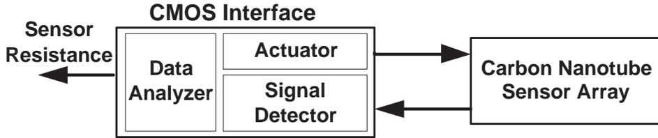
Figure 2-3: General concept of a sensor interface chip
