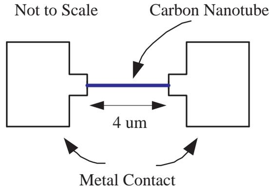
Figure 1-5: Simple CNT device with two metal contacts
