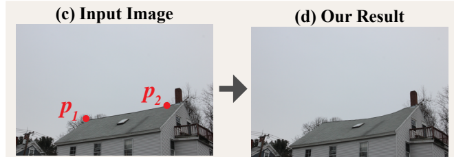
Figure 1: Revealing the sagging of a house’s roof from a single image. A perfect straight line marked by p_1 and p_2 is automatically fitted to the house’s roof in the input image (a). Our algorithm analyzes and amplifies the geometric deviations from straight, revealing the sagging of the roof in (b). View II shows a consistent result of our method (d) using another image of the same house from a different viewpoint (c). Each viewpoint was processed completely independently.
