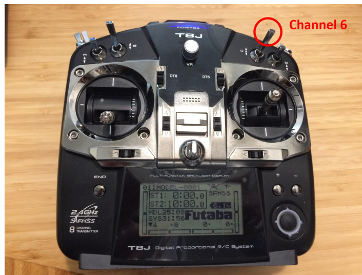
Figure 1: Channel 6 in our RC transmitter. It is a three-position switch but we only need two positions in this experiment.
