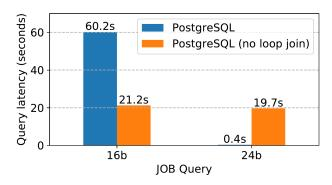
Figure 1: Disabling loop join in PostgreSQL can significantly improve (16b) or harm (24b) a particular query's performance. These example queries are from the Join Order Benchmark (JOB) [15].
