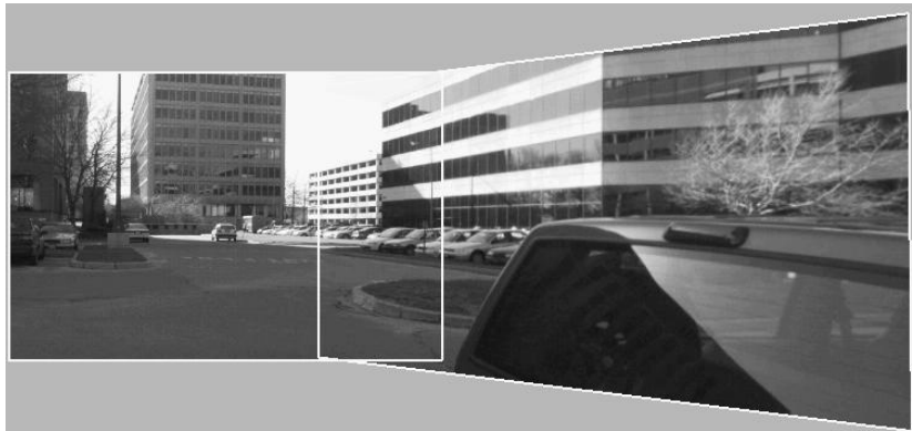
Figure 6: The projective warp between two images, after direct optimization.
