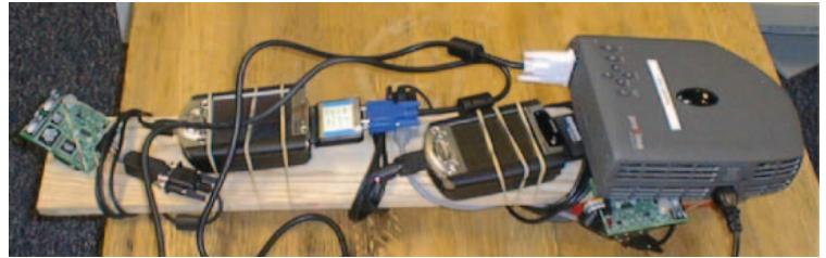
5 Prototype software flashlight. A software compass augmented with a PDA capable of image generation, and a compact digital projector.
