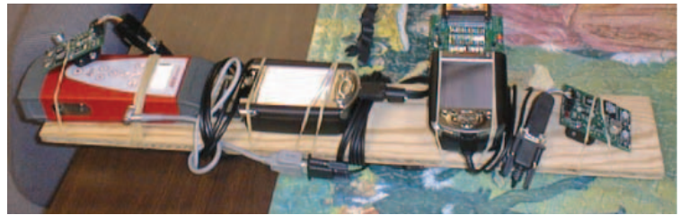
2 Prototype software compass. Two Cricket position listeners (at either end of board) separated by a fixed baseline and a handheld computer (center) fuse the position estimates into a single orientation estimate for the compass. A laser range finder is at the left.
