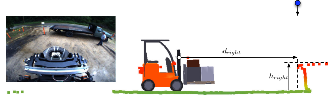
Fig. 7. Truck bed detection algorithm depicted on the raw data acquired from sensor mounted to the right of the mast.
