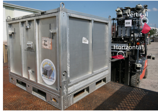
Fig. 2. The forklift detects pallets with a single horizontally-scanning LIDAR, and truck beds with a pair of vertically-scanning LIDARs.
