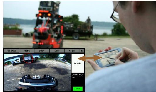
Fig. 3. Forklift being commanded, via the tablet interface, to pick up a pallet from a truck bed.
