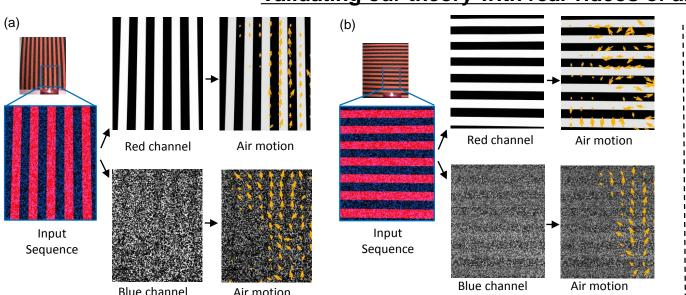
Hot air from a candle. Refractive motion estimation algorithm [4] fails if there is ambiguity. When the background structure is vertical (so that the air motion is parallel to the background), the recovered air motion is almost correct ((a) top). However, when the background structure is horizontal, the recovered air motion is incorrect ((b) top). The air motion estimated from fully-textured background serves a ground truth (bottom).
