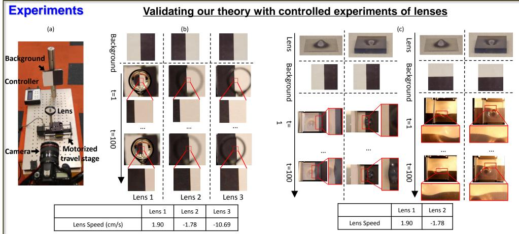
(a) Setup. (b) Illustration of the ambiguity when observing a first order structure. The same sequences are observed with in the aperture (red region), although three lenses move in different speeds. Thus we cannot recover the motion of the lens just from local observation. (c) Illustration of the ambiguity when observing a second order structure.
