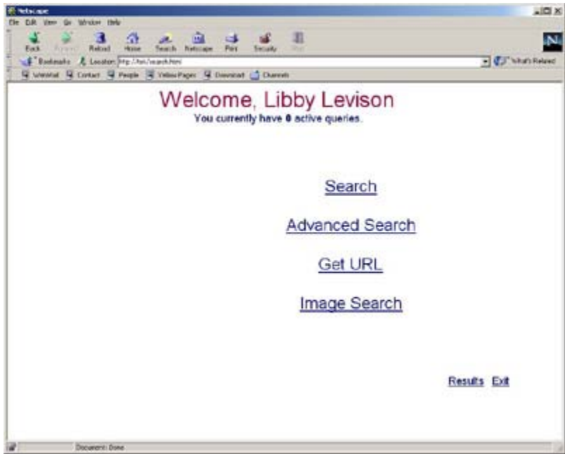
Figure 3: After logging in, the user can perform remote searches, including advanced search, specific URL request, and image search.
