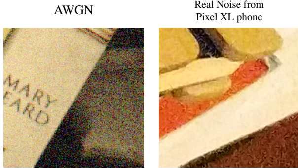
Figure 2: AWGN noise (left) and real noise from Pixel XL phones (right). The noise in real images is processed extensively by the camera pipeline. For this particular camera, the artifact is long-grained (right) and very different from the fine chroma pattern of AWGN (left).
