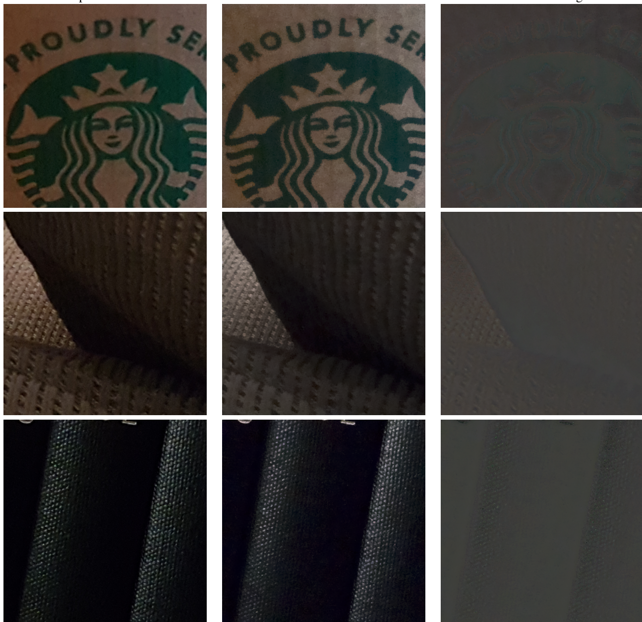
Matching Cellphone Camera Processing with Our Pipeline (Main Paper's Fig. 4): Samsung Galaxy S7 Simulation Cellphone's JPEG Our Simulation Difference Image
