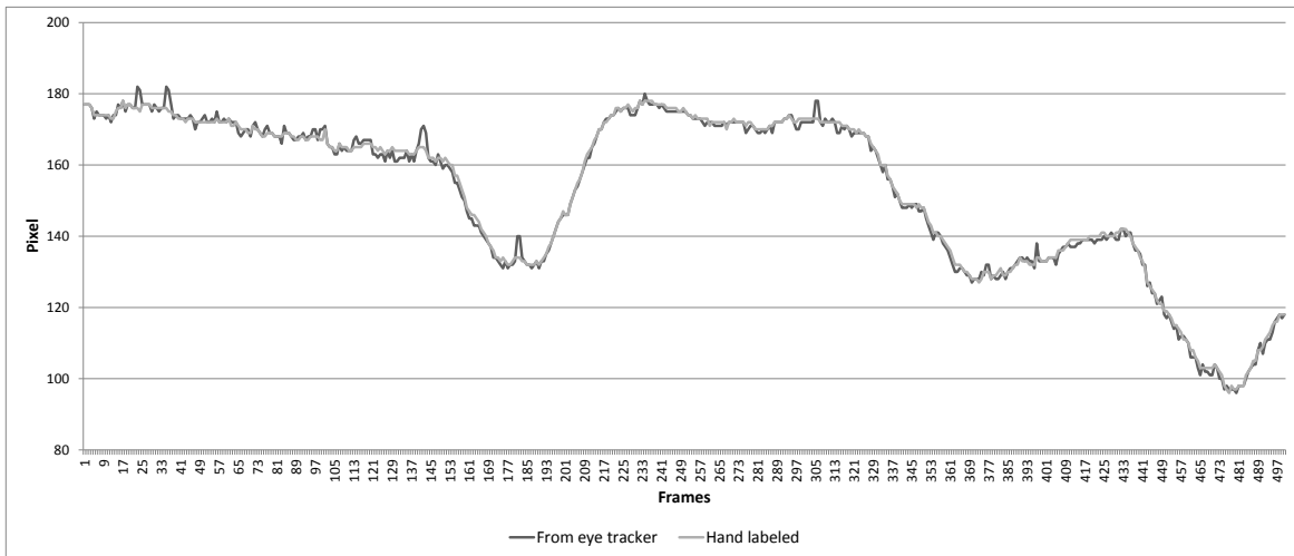
Figure 4.2: Tracked and Hand-labeled Right Eye (Row) Positions (Experiment 1)
