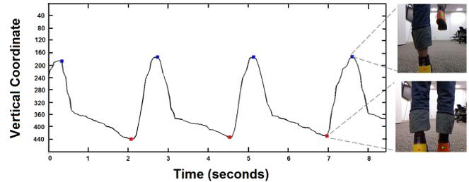
Fig. 5. This figure shows the detection of each event for one foot to show when a person’s foot is leaving the ground, and when their foot reaches its maximum height.
