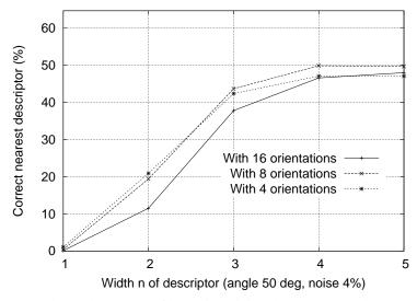
Figure 8: This graph shows the percent of keypoints giving the correct match to a database of 40,000 keypoints as a function of width of the  $n \times n$  keypoint descriptor and the number of orientations in each histogram. The graph is computed for images with affine viewpoint change of 50 degrees and addition of 4% noise.
