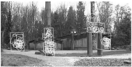
Figure 13: This example shows location recognition within a complex scene. The training images for locations are shown at the upper left and the 640x315 pixel test image taken from a different viewpoint is on the upper right. The recognized regions are shown on the lower image, with keypoints shown as squares and an outer parallelogram showing the boundaries of the training images under the affine transform used for recognition.
