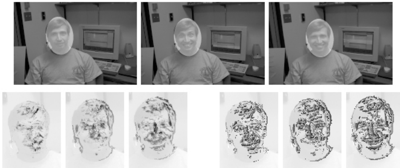
Figure 4. The adaptation of the model during tracking. (top) The target region in selected frames 200, 300, 480. (bottom) The stable component's mixing probability (left) and mean (right) for the selected frames.
