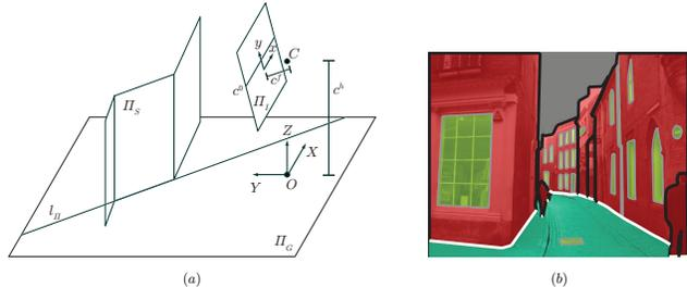
Figure 2. (a) Camera and scene layout. A scene is composed of objects, represented as piecewise-connected planes, standing on a ground plane. (b) Polygon and edge types. Polygons are either *ground* (green), *standing* (red), or *attached* (yellow). Edges are *contact* (white), *occluded* (black), or *attached* (gray).
