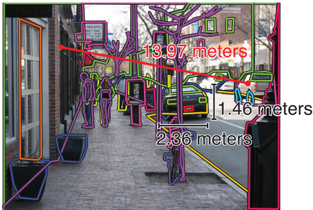
Fig. 7. Snapshot of the 3D measuring tool. Once we compute the 3D coordinates for a depicted scene, we can make measurements of scene components. Here, we show the height and width of the car, which is 13.68 meters away from the camera center. We can also compute the distance between any two points in the scene, such as the selected points on the building and the truck.
