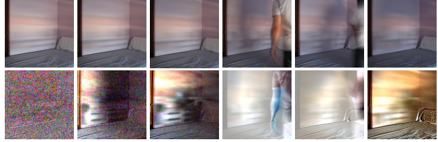
Figure 9. top row) Input sequence (a person walks inside a room moving toward and from a window not visible in the movie), bottom row) difference between reference image (first frame of the video) and each frame. The difference creates an approximation to a camera obscura with an aperture that moves as the occluder moves inside the room (see companion video).
