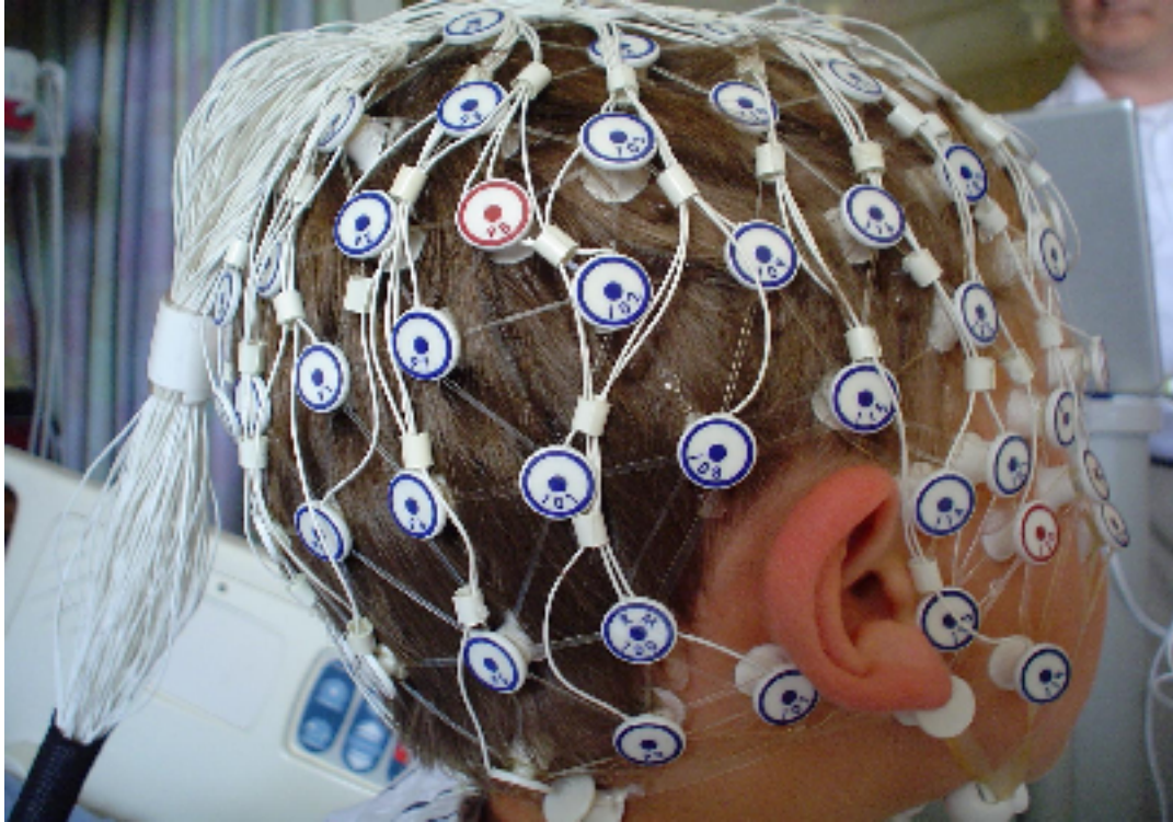
Figure 2-3: 128-channel Surface EEG. The electrodes are applied as a grid providing for a more systematic placement of electrodes. The larger number of EEG channels also provide for higher spatial resolution.
