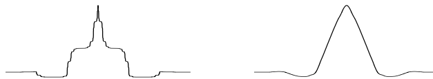
Figure 3. An example why non-uniform subdivision is needed. Left the limit function with uniform subdivision, right non-uniform. The same irregular grid is used in both figures.
