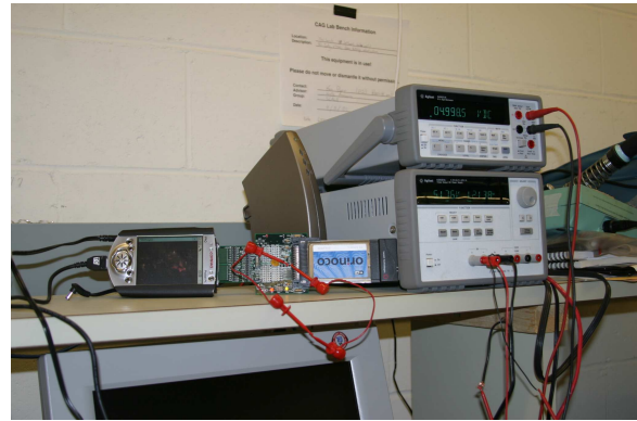
Figure 6: Our experimental setup for measuring the power consumed by an iPAQ and the wireless network card.
