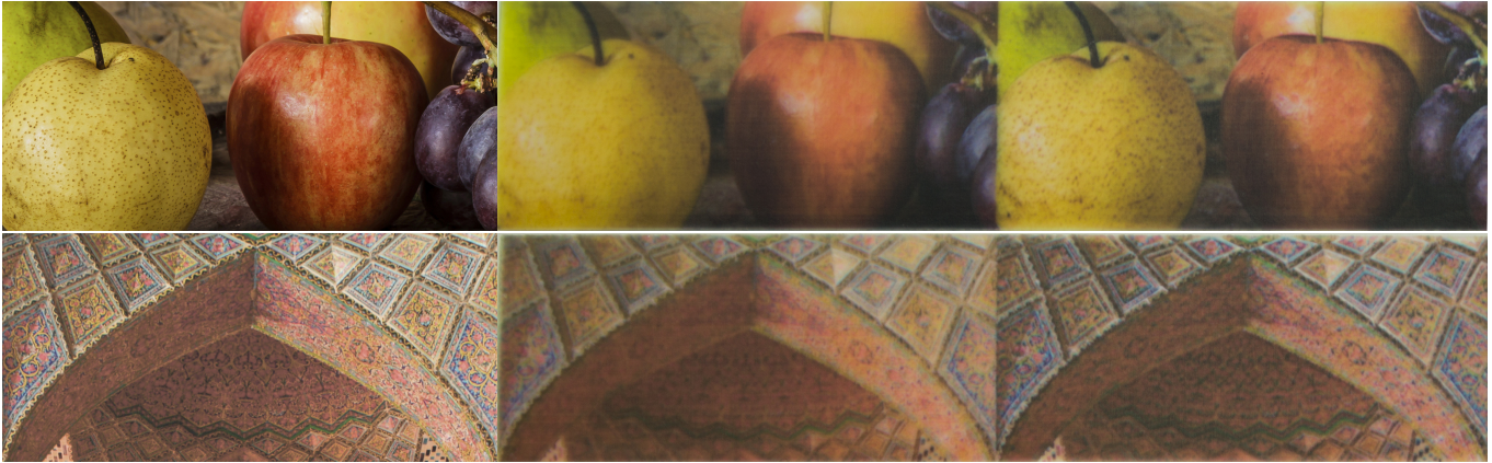
Fig. 15. Left: The original image (gamut mapped). Middle: Photograph of the print of the original image with standard contoning. Right: Photograph of the print of the presharpened image. The estimated blur kernel is a Gaussian with filter size 30 XY-voxels and standard deviation 10, estimated from a blur calibration print.
