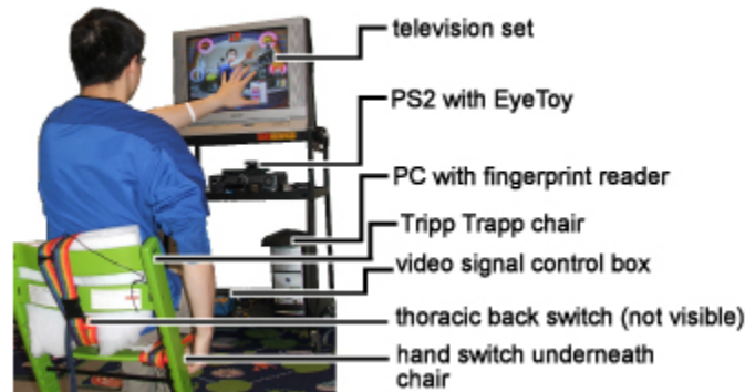
Figure 3.1: Photograph of system setup. The participant sits approximately six feet away from the screen and “reaches” for virtual objects visible on the TV.
