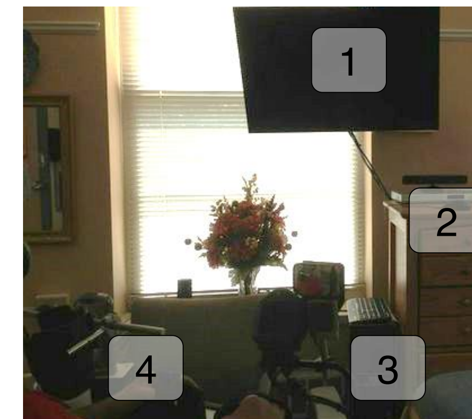
Actual bedroom setup with 1) television, 2) Kinect, 3) computer, and 4) wheelchair with voice activated remote control
