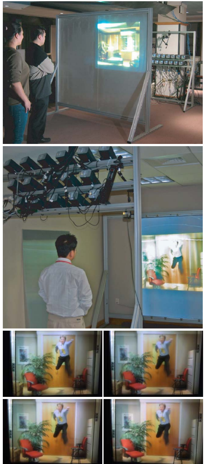
Figure 1: Our 3D TV system with a rear-projection display (first row) and a front-projection display (second row). Images of a scene from the viewer's side of the display (third and fourth row).
