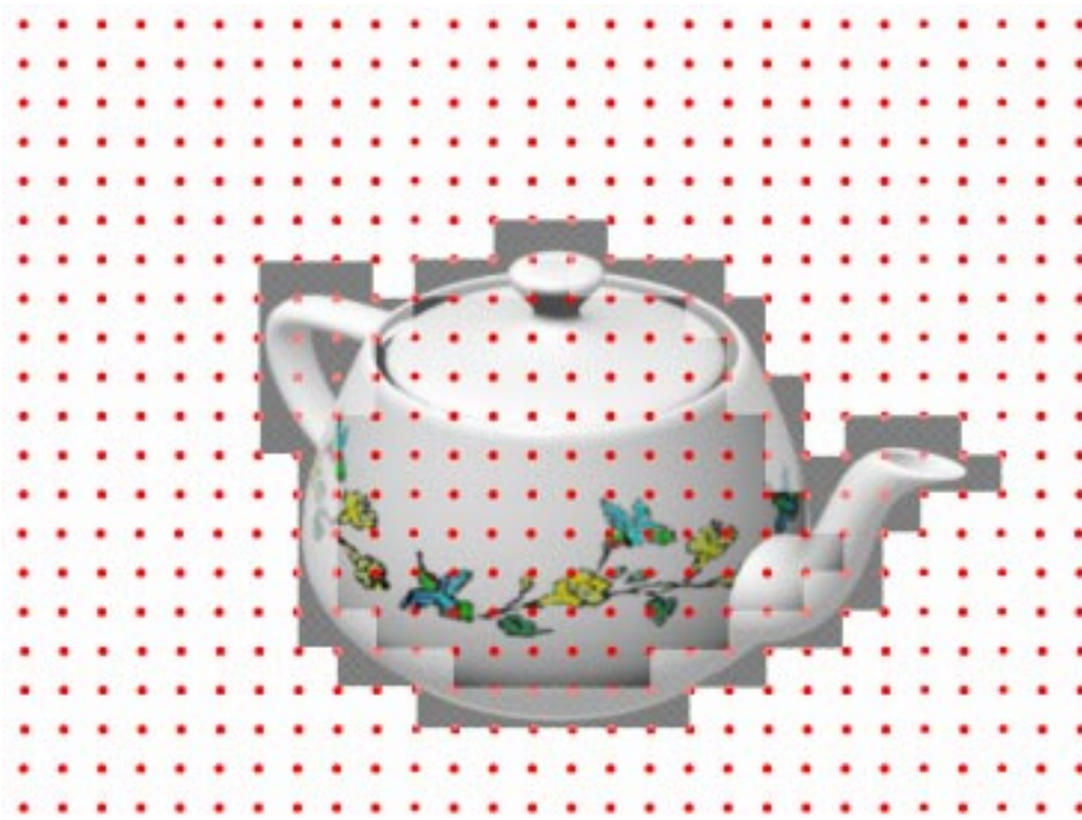
Figure 3.9 Coarse-to-Fine Sampling. In the first pass one samples at low resolution (red dots). In the second pass one samples at high resolution but only on the visual hull boundary.
