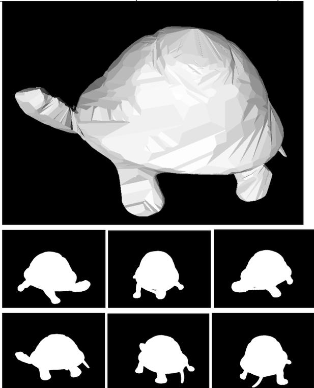
**Figure 3: Shaded image of the visual hull and 6 out of 26 input silhouettes that generated it.**
