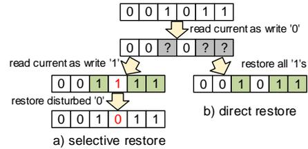
**Figure 4: Comparison between the previous restore operation and our fast-restore operation**
