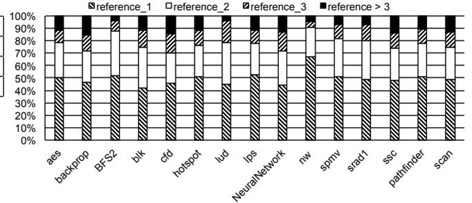
**Figure 2: Register read access count distribution. It shows the number of read accesses to registers.**
