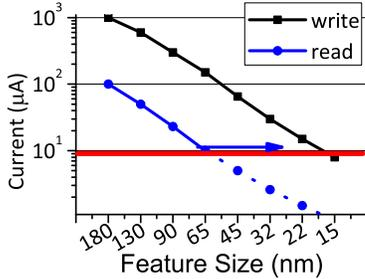
**Figure 1: The scaling of read and write currents [17]**
