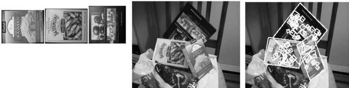
Figure 2-13: An example of object recognition from local scale-invariant features [77]. Model images of planar box faces are matched in a cluttered scene containing occluded objects. The SIFT approach successfully discovers these objects.
