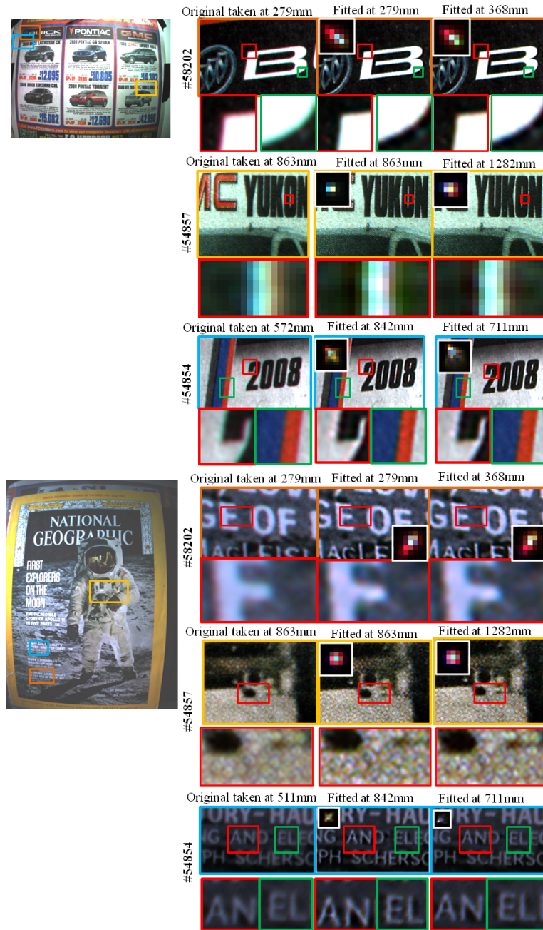
Fig. 12: Image enhancement results of a newspaper and a National Geographic magazine cover. We take a image (first col.), and fit lens prescriptions at two different depths, respectively, and use them to enhance the image (second and third col.). The insets show reduced aberrations and chromatic aberrations.
