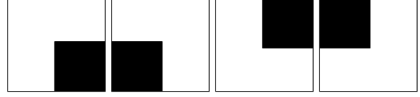
Figure 6: Four templates used for corner detection in our system.
