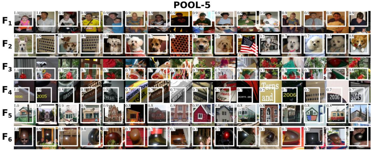
Figure 2.8: Illustration of the visualizations reported in [82]. They displayed, a set of 96 images, where each line represents the max-16 images that highly activate a filter. In each max-image, they highlighted (in a white window) the region that highly activate the actual filter. In their paper, they only visualized 6 filters of the last pooling layer ( pool – 5) of AlexNet, which thus corresponds to filters of the las convolutional layer ( conv – 5). Best view in color.
