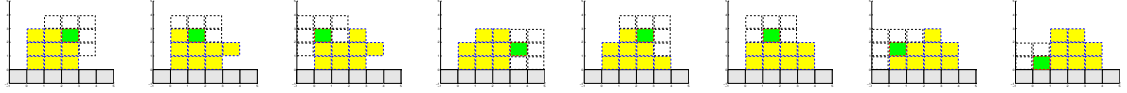
Fig. 4. Snapshots of a manually-driven sequence for 3x3 modules. Green modules are selected by an operator. Dotted regions denote the possible next locations.
