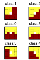
Fig. 6. Superposed support vectors. The yellow blocks denote empty and the brown is a robot or an obstacle. The white blocks are not included in the classifiers.
