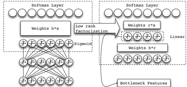
Fig. 1. Diagram of the low-rank factorized DNN.
