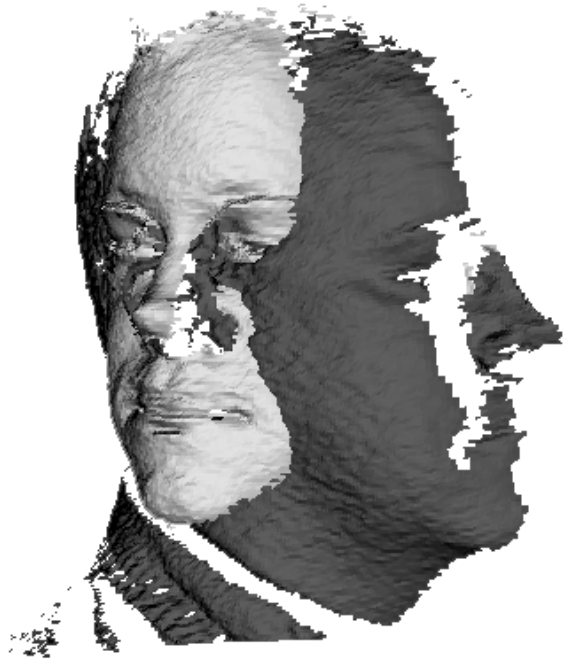
Figure 2: Rendering that demonstrates a catastrophic failure of the registration when large non-overlapping regions exist and no corresponding point pairs are classified as outliers
