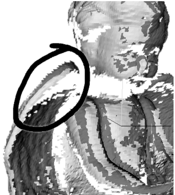
Figure 3: Rendering that demonstrates a mis-registration at the edge of the wing in the circled region.
