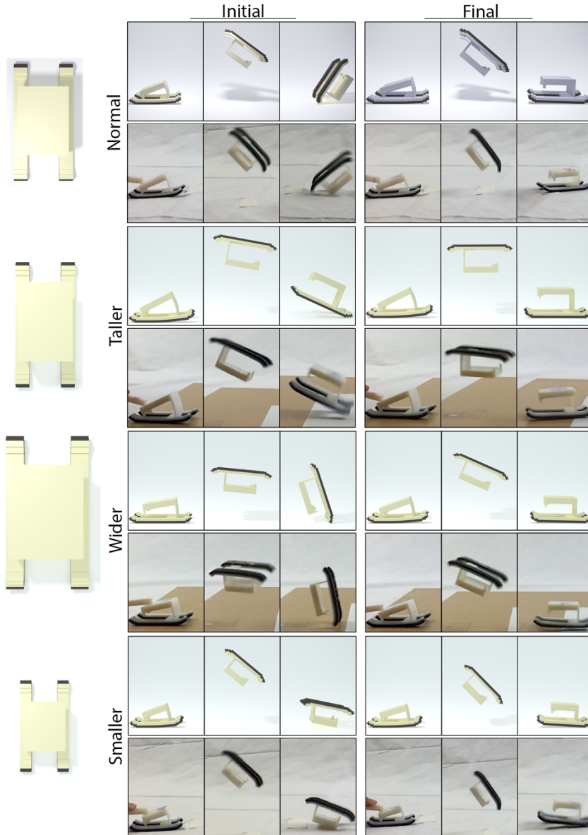
Figure 4-25: A comparison of experimental (bottom) and DAC/BBI simulated (top) results for six more design samples: initial (left) and final (right) designs of variations on the flipping mechanism (“Normal”).
