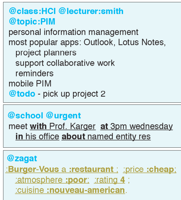
Figure 2. Jourknow supports combinations of tags and unstructured text (top), pidgin grammars (middle), and Notation3 (bottom).
