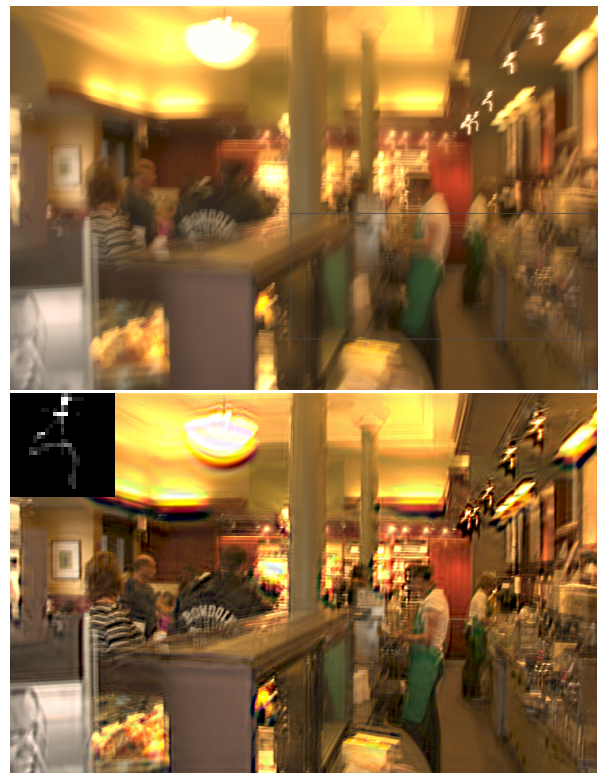
Figure 13: Top : A blurred scene with heavy saturation, taken with a 1 second exposure. Bottom : output of our algorithm.
