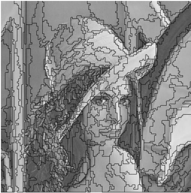
Figure 3: Partitioning of 512 \times 512 image by evolution with 500 ranges (compression ratio 70.5). Shape information = 2029 bytes, transformation information = 1691 bytes.
