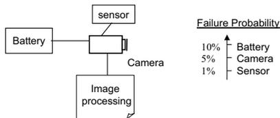
Figure 1: Camera Module for Navigation System
