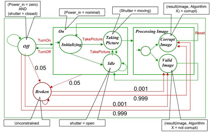
Figure 4: PHCA model for the camera/image processing module. Circles represent primitive locations, boxes represent composite locations and small arrows represent start locations.
