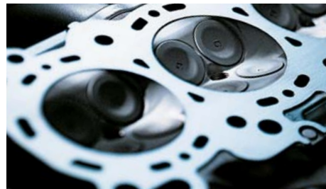
4 valves per cylinder for easy breathing.
