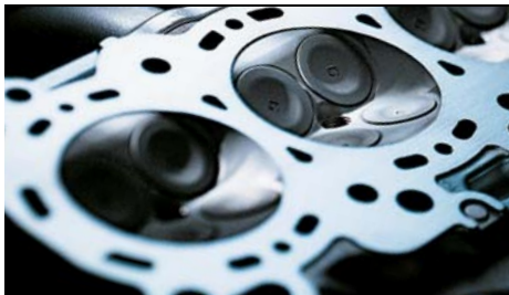
The 4-valve design makes the flow really go.
